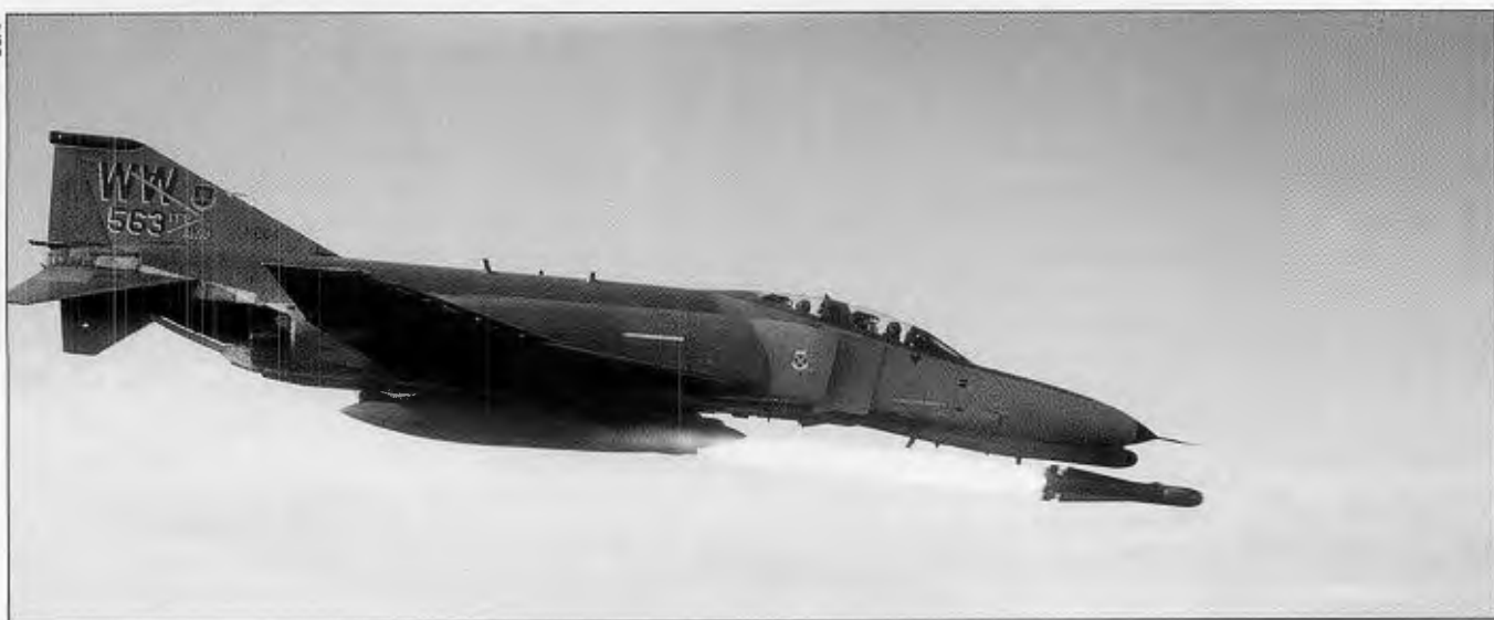
An F-4E Phantom II aircraft of the 37th Tactical Fighter Wing launches an AGM-65 Maverick missile.
